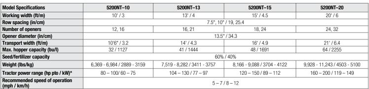
Pull-type rigid frame — hydraulic weight transfer tongue — dual wheels — fluted, coulters indexed to openers — Precision Residue Opener — rotary scrapers — front mounted transmission drive system — easily adjustable seed cups — digital acre meter — treadwalk - LED lights — dry fertilizer meter and drive, press wheels, row markers
