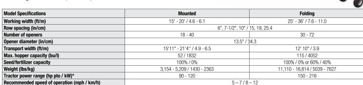
3-pt or drawbar hitch with hydraulic tongue — walking tandem mainframe wheels on folding models — Precision Residue Opener — rotary scrapers — front-mounted transmission drive system — easily adjustable seed cups — digital acre meter — treadwalk - LED lights — dry fertilizer meter and drive on folding models, press wheels, row markers
